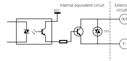
In the figure above, **V-** is the common terminal of external output signal and **OUT** is the output signal.
